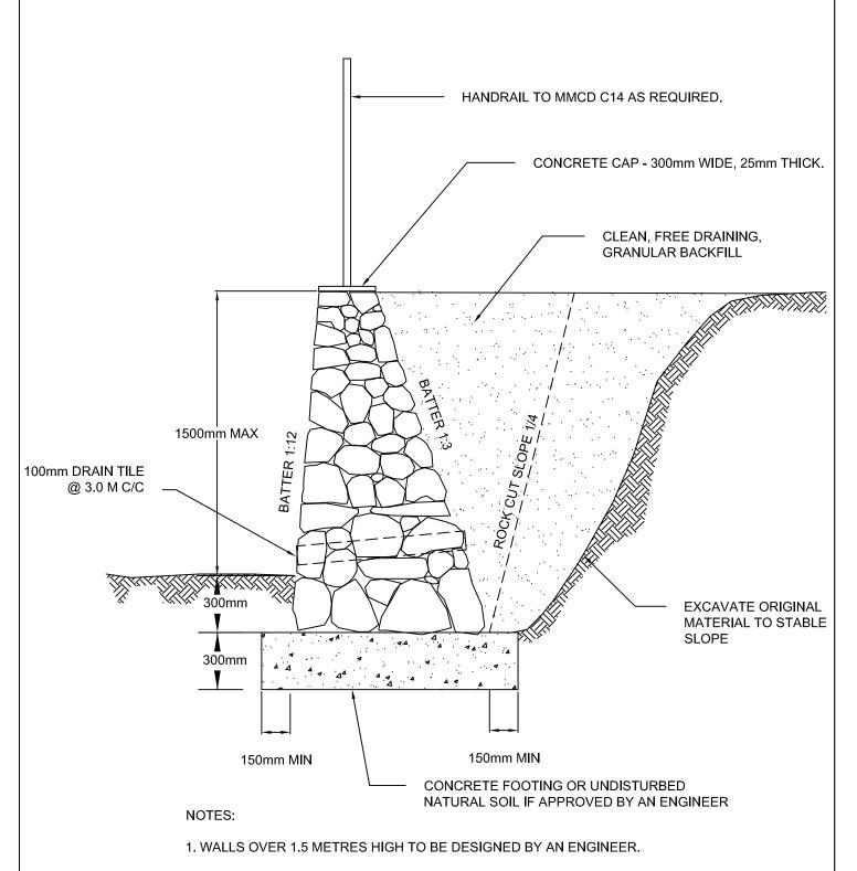
2. MORTAR TO BE 1 PART PORTLAND CEMENT TO 2 PARTS SAND.
