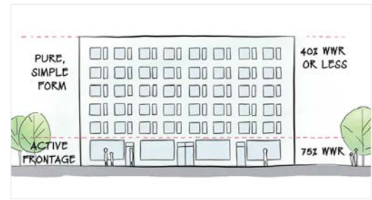
Figure 29: While retaining at-grade transparency, targeting lower window-to-wall ratios on building elevations can significantly reduce energy demand. As general guidance, designers targeting the Lower Steps of the Step Code should target no more than a 50% WWR and designers targeting the Upper Steps should target a WWR of less than 40%.
