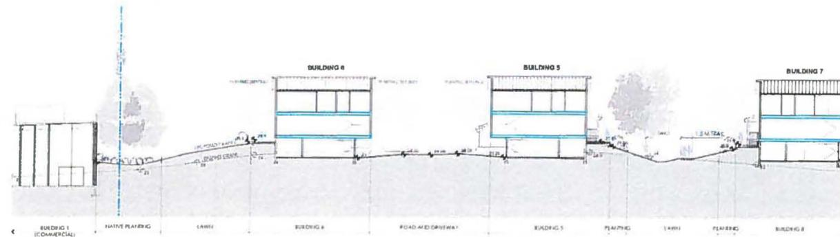
SECTION BB - SCHEMATIC SECTION THROUGH BUILDINGS 1, 5, & 7
