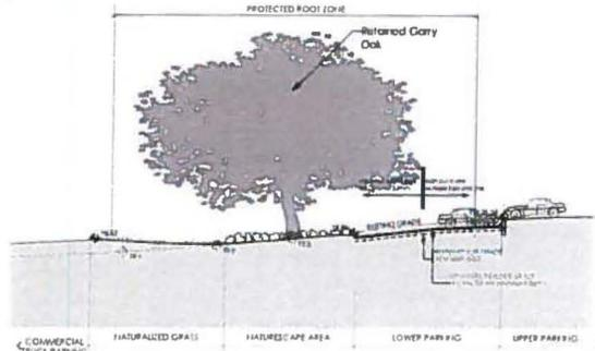
SECTION CC - SCHEMATIC SECTION THROUGH EXISTING GARRY OAK #605 TO BE RETAINED
