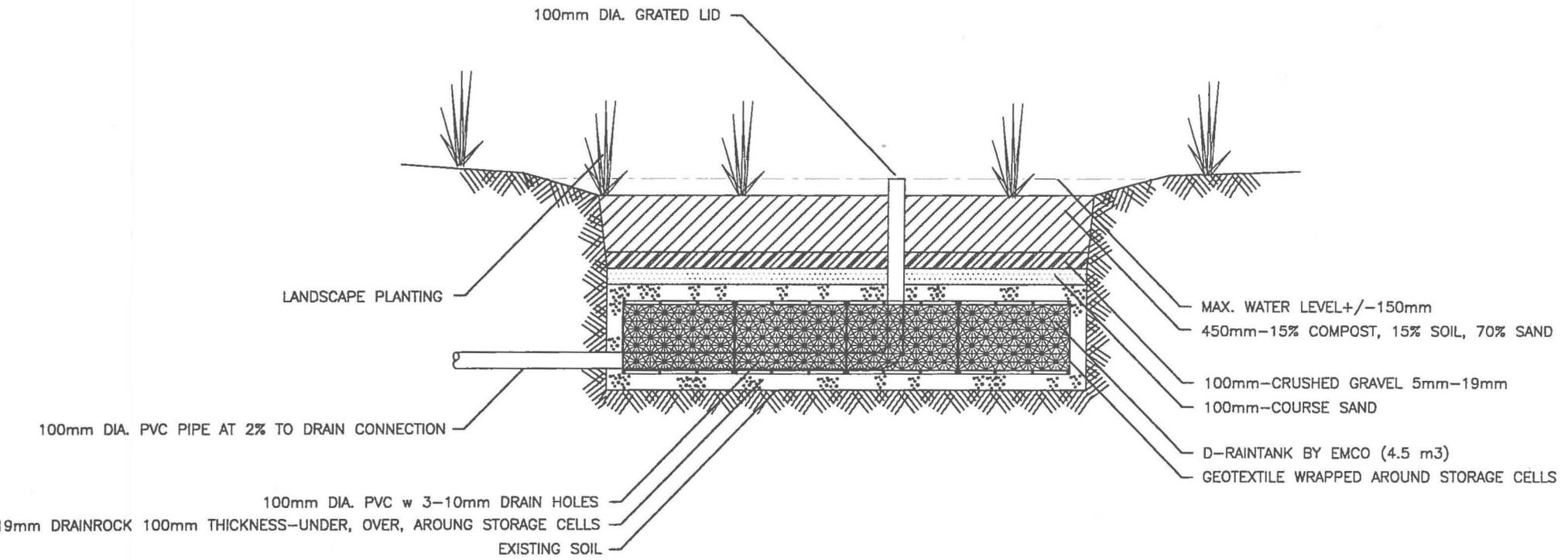
**Figure 4: RAIN GARDEN TREATMENT/DETENTION – DETAIL**
