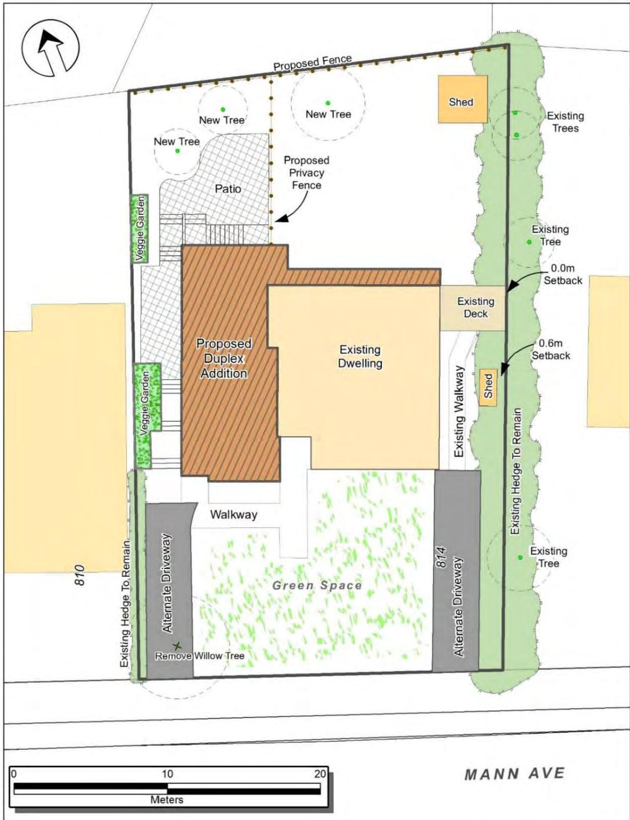
Figure 7: Example of an Alternative Parking Configuration
