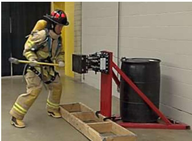
Starting from a standing position, you will pick up the 4.5 kg (10 lb) sledge hammer and use it to strike the mechanically-braked target surface of the forcible entry apparatus.
