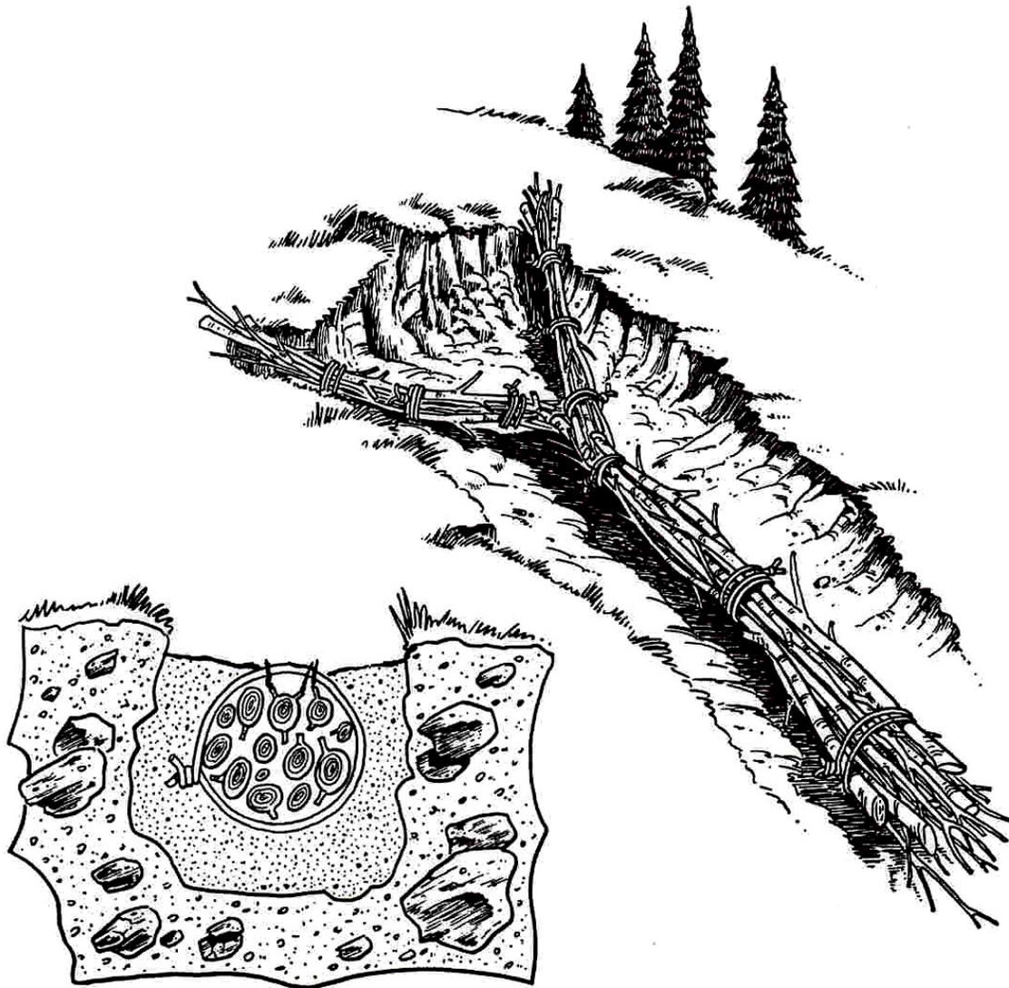
**Figure 2.** Live pole drains are bundles of cuttings that provide a preferred flow path for soil moisture.
