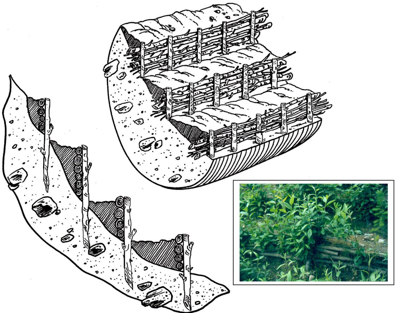
**Figure 1.** Wattle fences are short retaining walls built of living cuttings. Both the stakes and the horizontal pieces will sprout and grow (inset) providing a dense growth of pioneering species on the slope.
