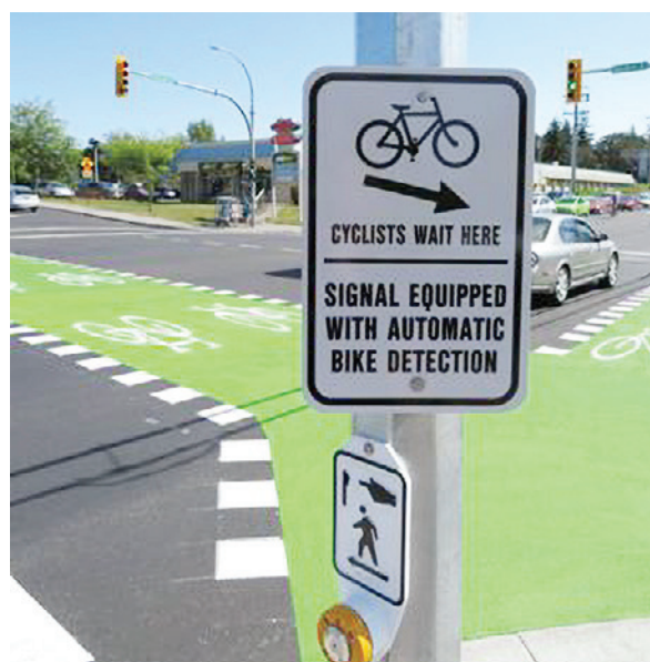
McKenzie Avenue and Borden Street bidirection bike lane crossing. This photo highlights automatic bike detection at the crossing.
