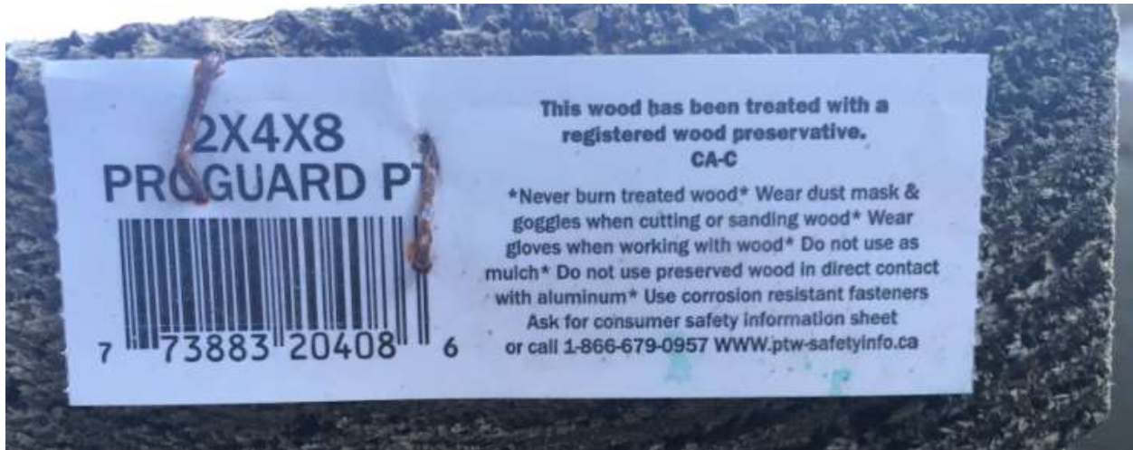
Figure 4 Warning Label on Residential Lumber treated with Copper Azole at Major Building Supply
