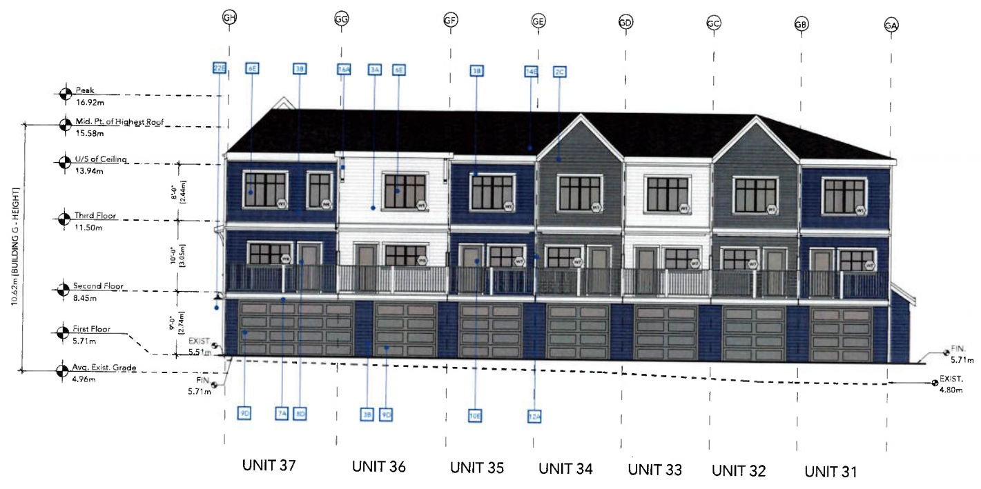
1 BUILDING G - NORTH ELEVATION DP-25 SCALE: 1:100
