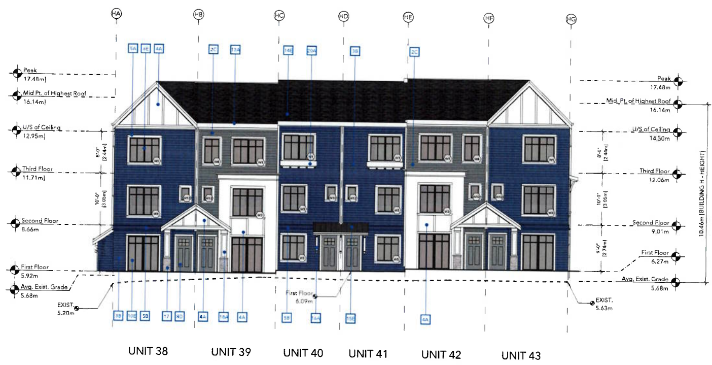
3 BUILDING H - SOUTH ELEVATION DP-26 SCALE: 1:100
