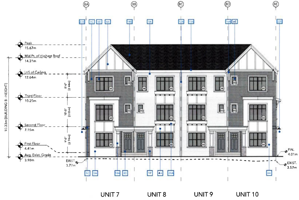
3 BUILDING B - SOUTH ELEVATION DP-20 SCALE: 1:100
