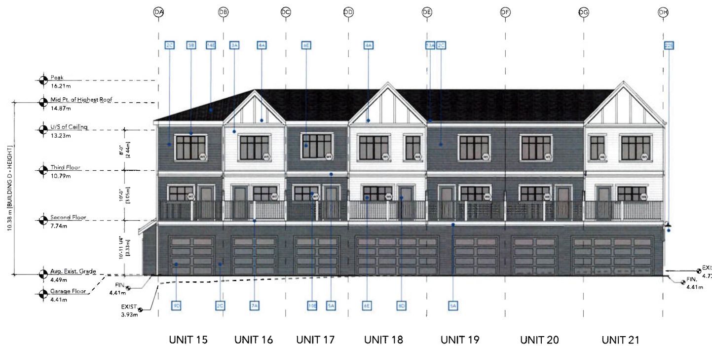
3 BUILDING D - SOUTH ELEVATION DP-22 SCALE: 1:100
