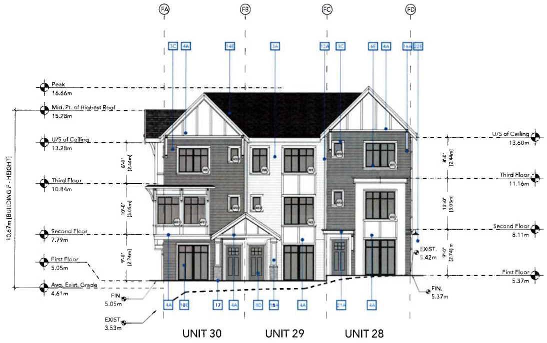
2 BUILDING F - EAST ELEVATION DP-24 SCALE: 1:100
