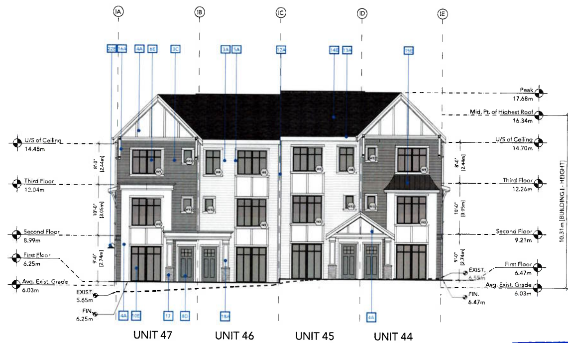
2 BUILDING I - EAST ELEVATION DP-27 SCALE: 1:100
