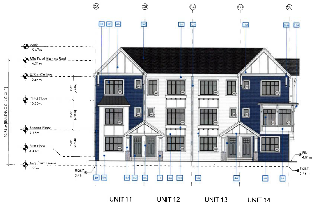
3 BUILDING C - SOUTH ELEVATION DP-21 SCALE: 1:100
