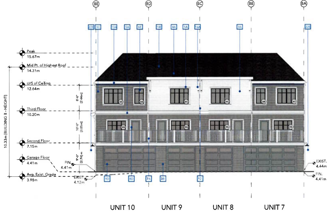
1 BUILDING B - NORTH ELEVATION DP-20 SCALE: 1:100
