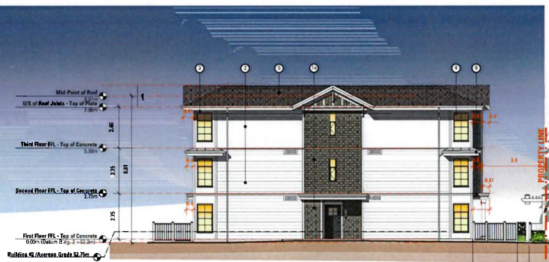
2 Apartment Building 2 - North Elevation SCALE: 1:100
