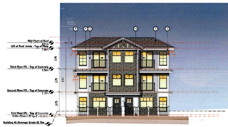
3 Apartment Building 2 - East Elevation SCALE: 1:100
