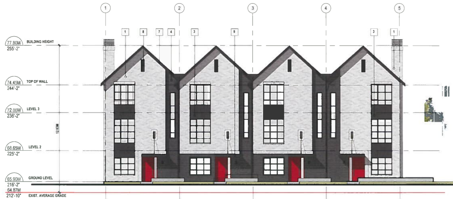
1 SOUTH-EAST ELEVATION Scale: 1/8" = 1'-0"
