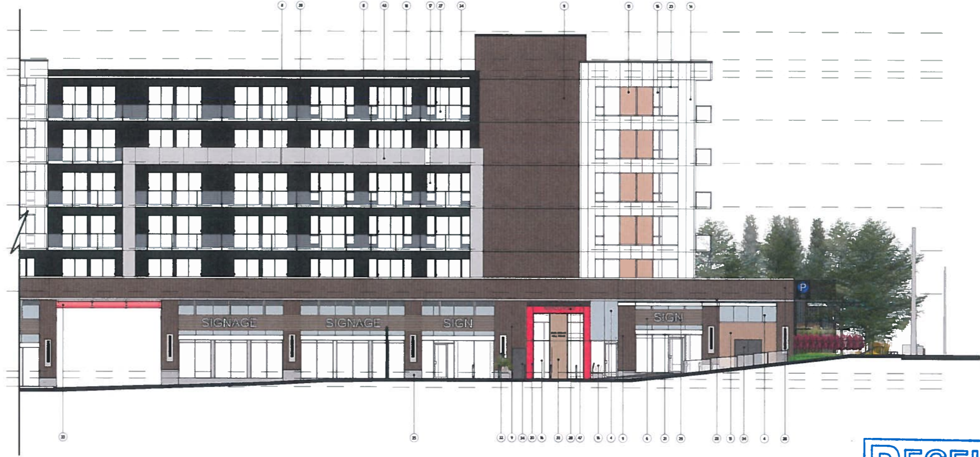
1 BUILDING A - PARTIAL NORTH ELEVATION ASB 1/8" = 1'-0" (1:304)
