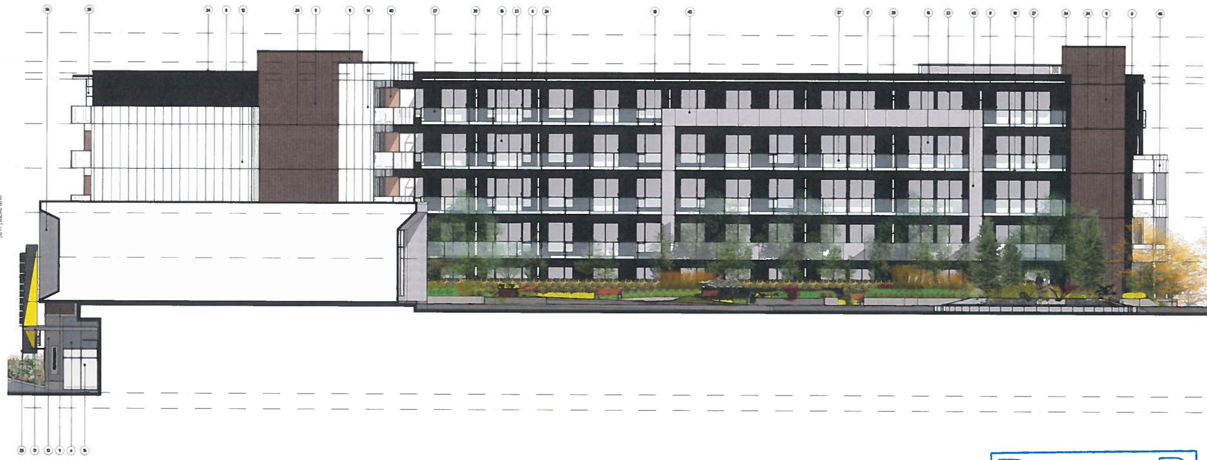
1 BUILDING B2 - EAST ELEVATION (COURTYARD) 4315 1/8" = 1'-0" (1:8)
