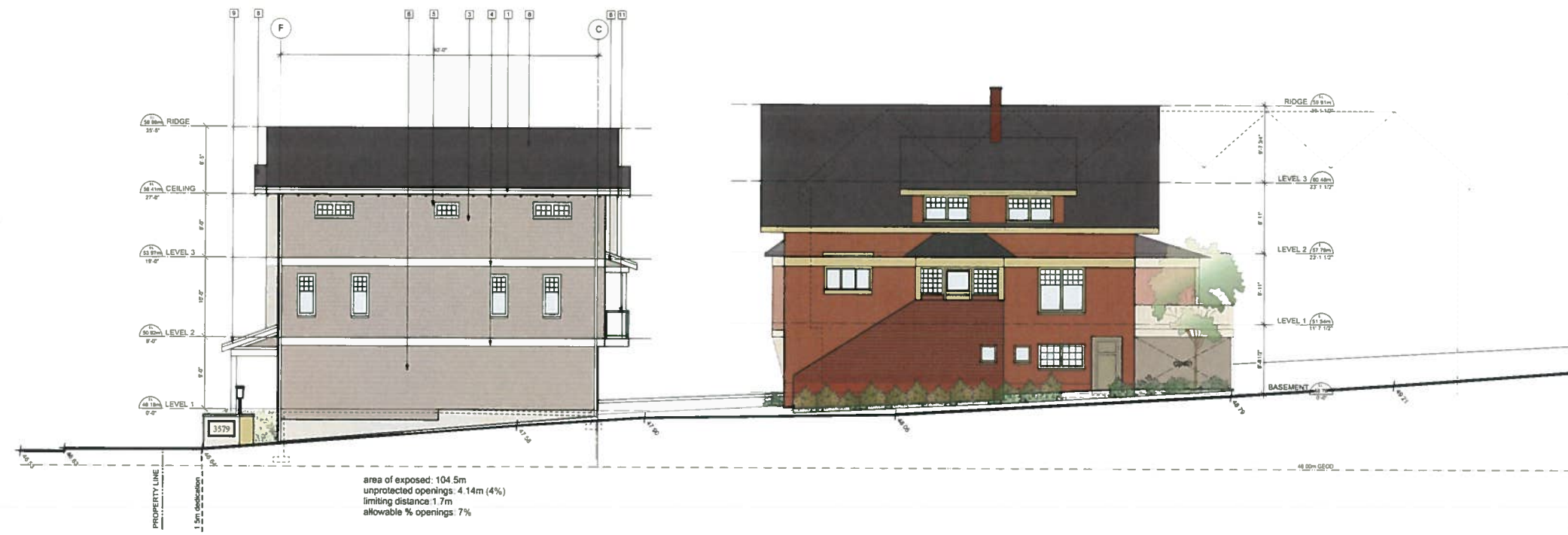
2 SOUTH ELEVATION - UNITS 2 + EXISTING HOUSE SCALE: 1:100
