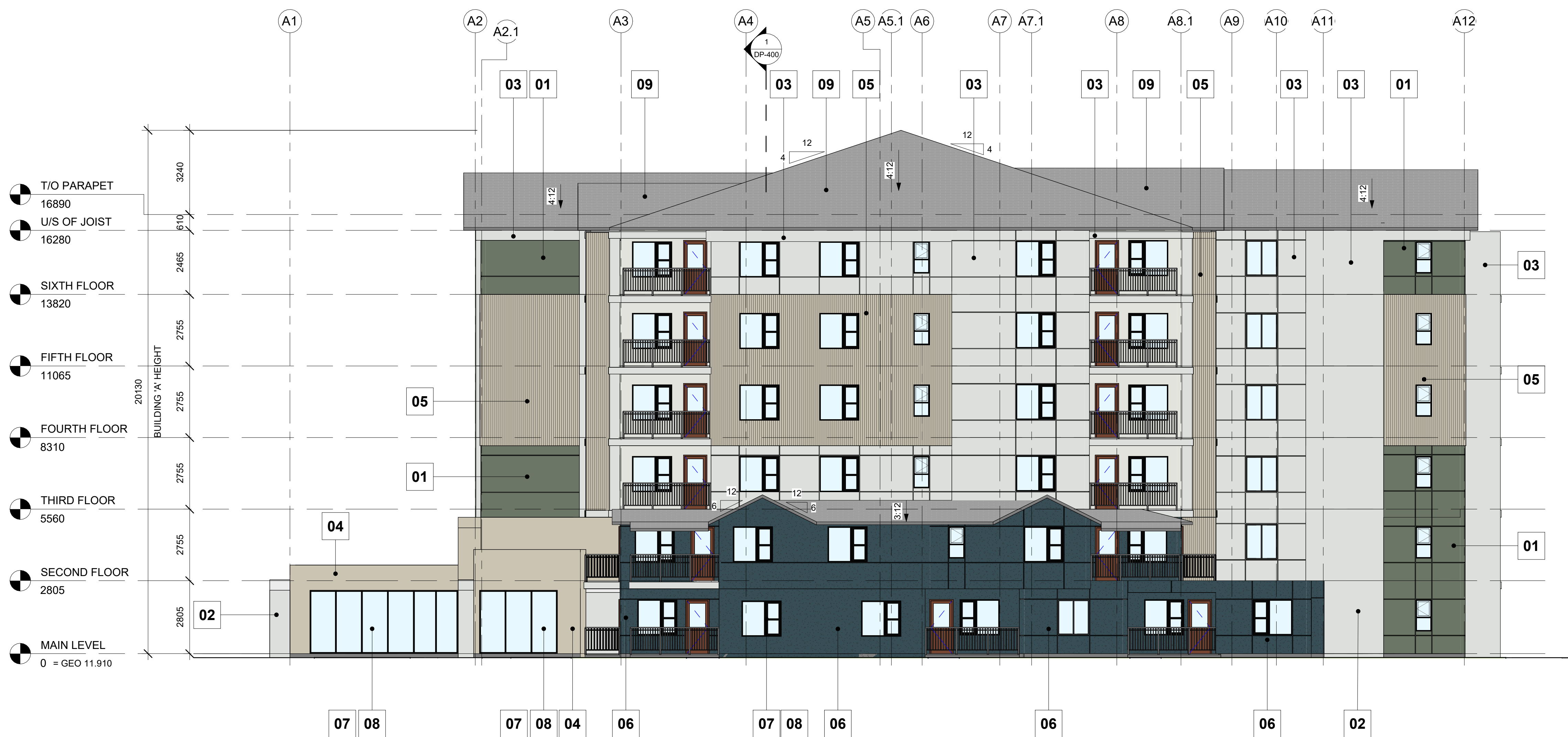
2 DP-301 BUILDING A WEST ELEVATION SCALE: 1: 100
