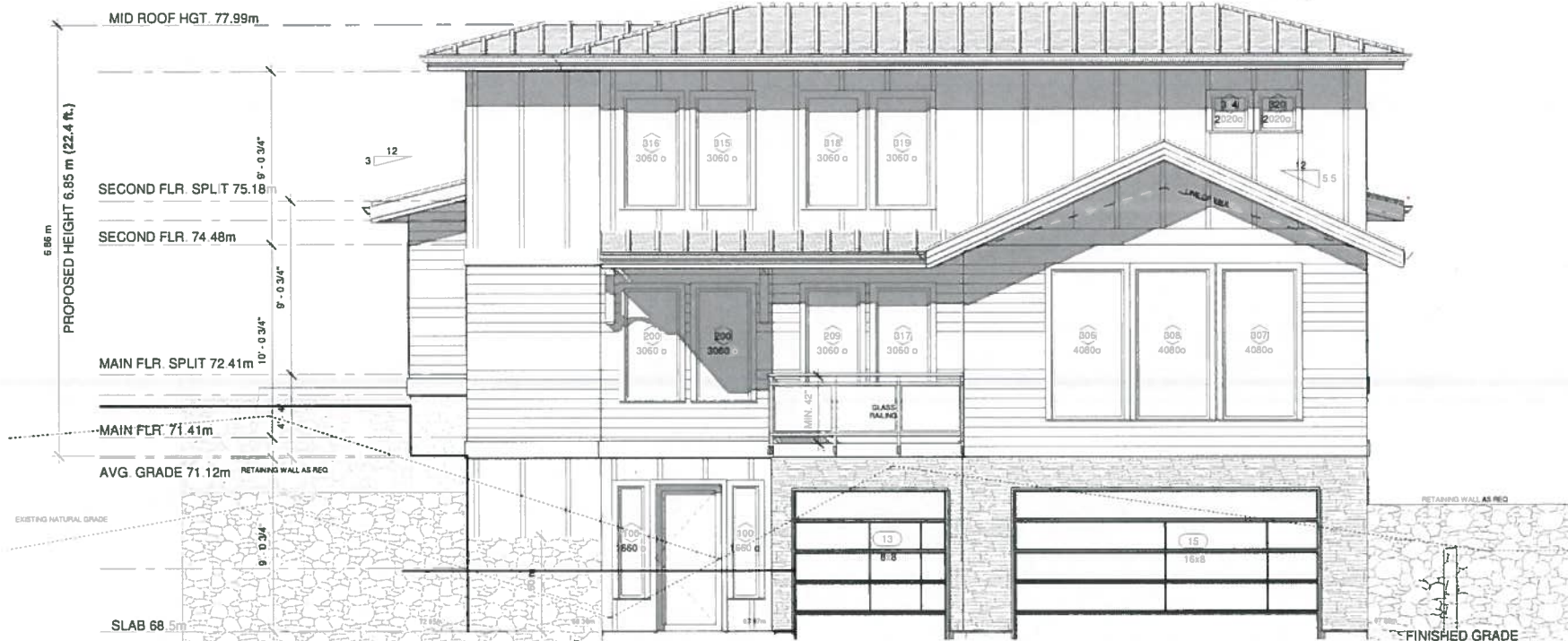
1 Front (north) Elevation 1/4" = 1'-0"
