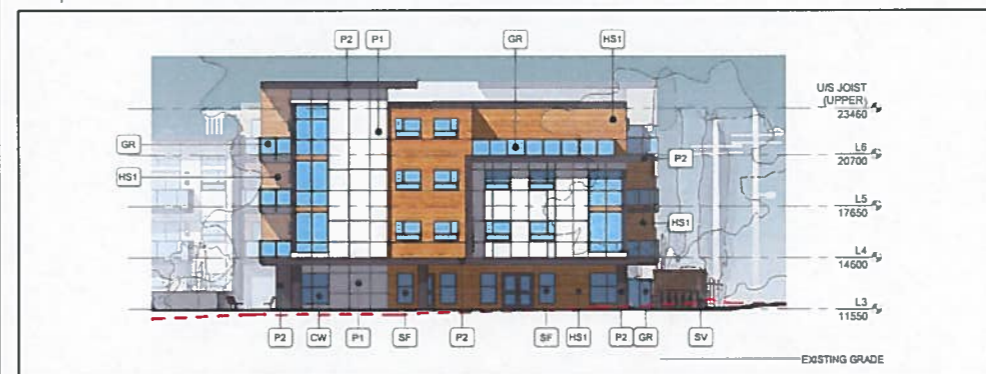
5 | EXTERIOR ELEVATION - NORTH (BLDG B) 1:200
