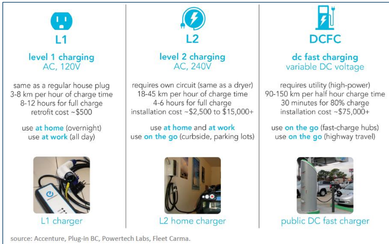
Figure 8: Different kinds of EV charging infrastructure.
