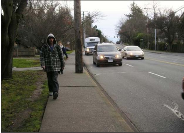
Pedestrians walk along the inside edge of sidewalk because there is no buffer from traffic. Note the path in the grass worn by walkers seeking greater distance from the street.
