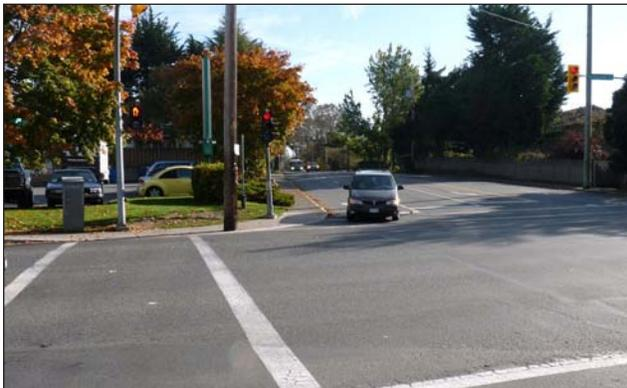
The rounded corner at Feltham and Shelbourne encourages traffic to turn without stopping and is dangerous for pedestrians, who have little space on the sidewalk to stand back from traffic.
