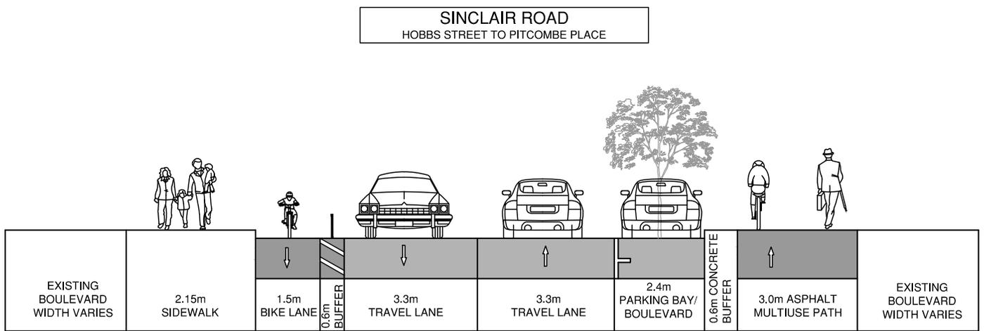
Figure 6.3: Sinclair Road Design Concept- Middle Section (Segment 2)
