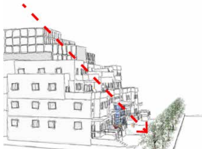
Figure 9.8: Mid-Rise development showing 45° angular plane
