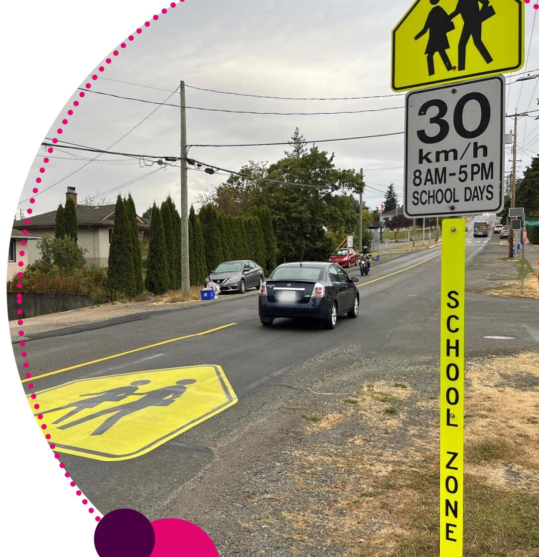
Enhanced school zone safety features were recently installed at a number of Saanich schools to reinforce 30 km/h speed limits.
