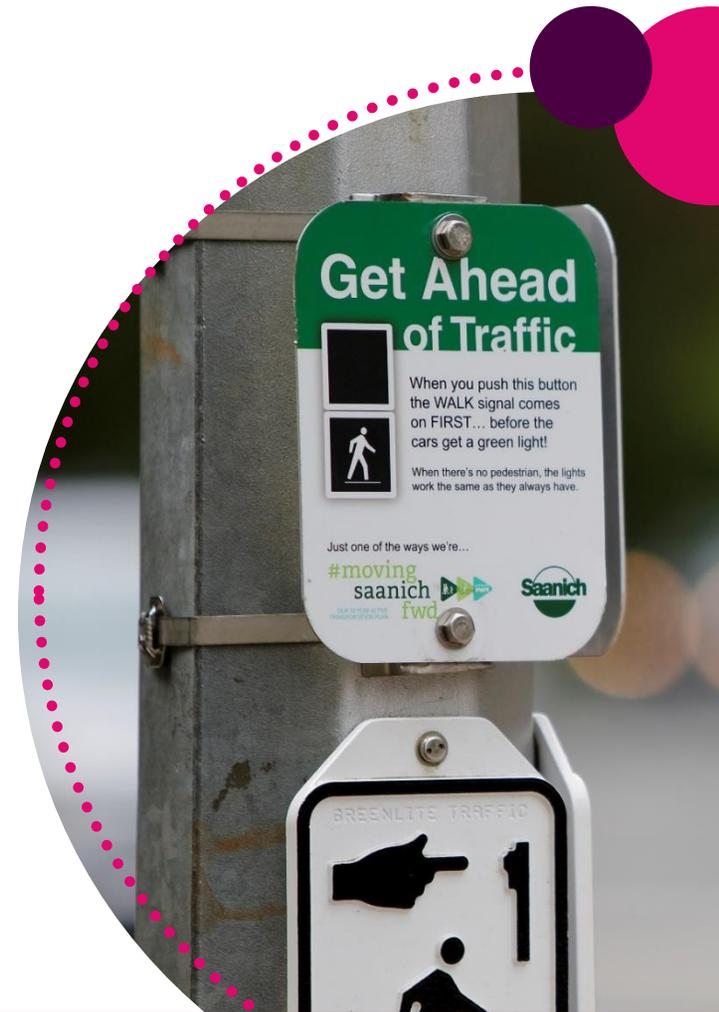
A **leading pedestrian interval (LPI)** gives pedestrians a head start when entering an intersection to enhance visibility and reinforce their right-of-way over turning vehicles
