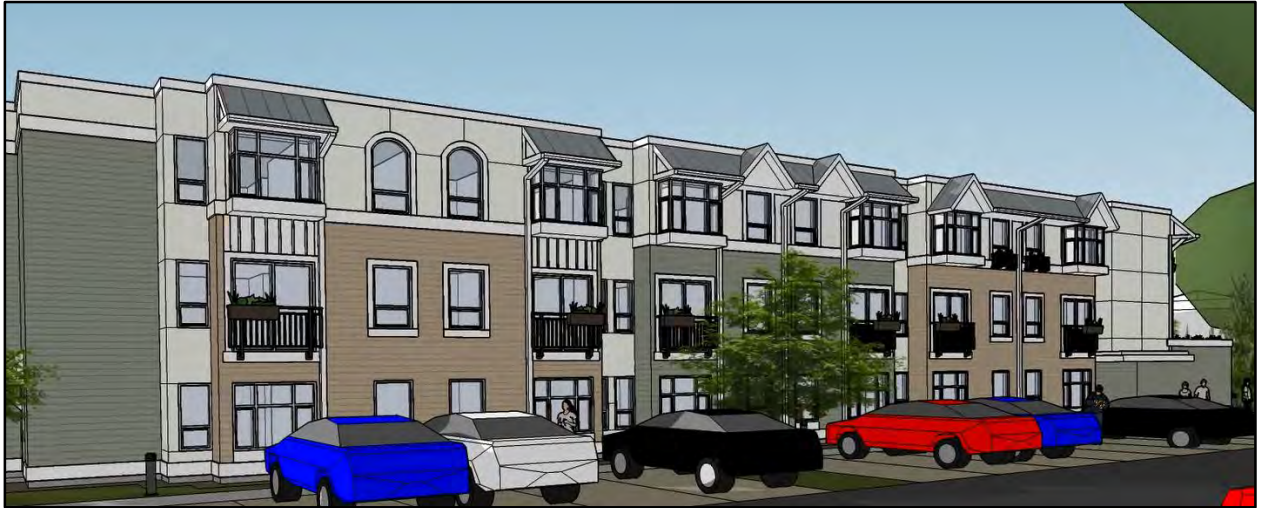
Figure 11: East Elevation – Juliette balconies and Bay Windows
