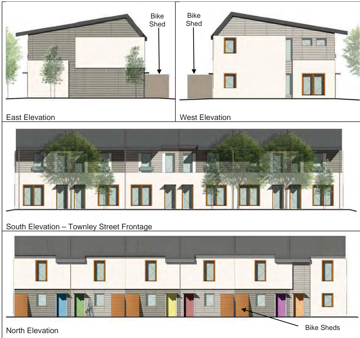
Figure 7: Two Storey Townhouse Elevations
