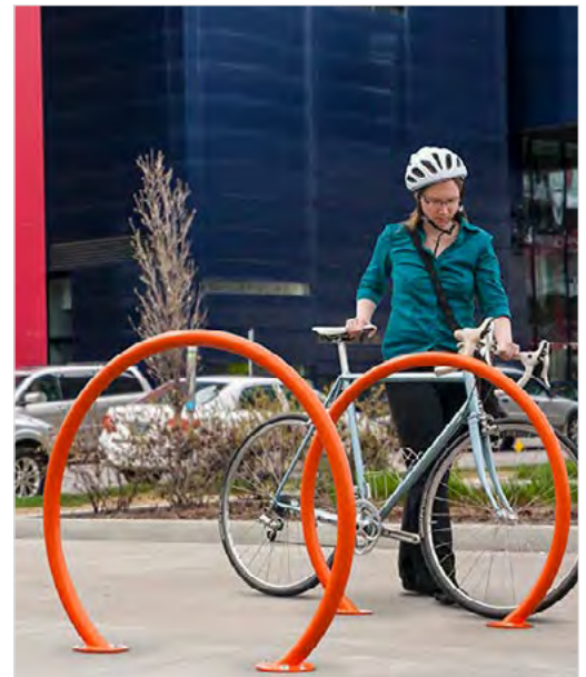
Figure 36: Bicycle rack able to support a bike in an upright position with at least two points of contact (3.4.2 a).
