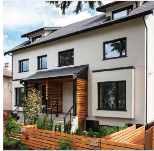
Figure 27: An example of a high-performance townhouse with a simplified building form to minimize building envelope heat loss, while also achieving many form and character objectives. (3.3.1. a).
