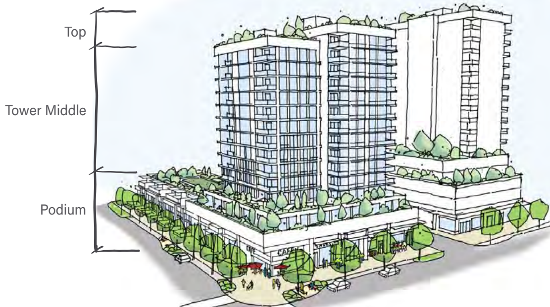
Figure 97: Design tall building to have a distinct podium, tower, and top (7.1.6. a).
