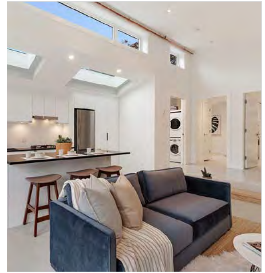
Figure 143: Natural light through clerestory windows improves livability.
