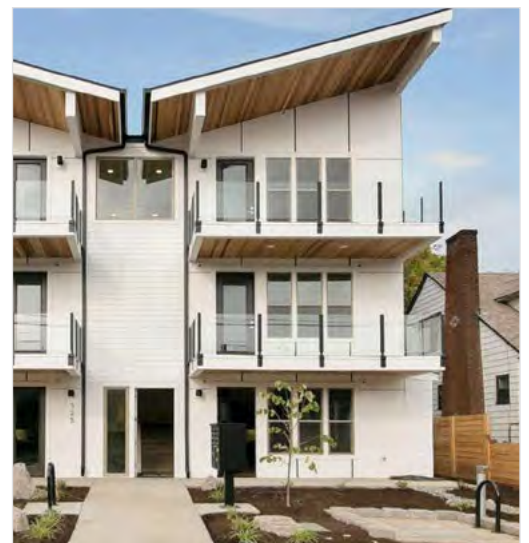
Figure 59: All units should be provided with windows of sufficient size and orientation to provide sunlight and outward views (4.1.6 d).
