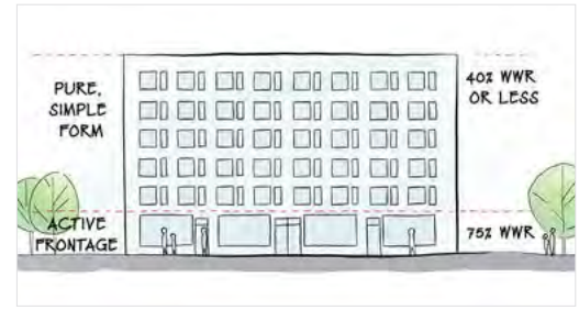
Figure 29: While retaining at-grade transparency, targeting lower window-to-wall ratios on building elevations can significantly reduce energy demand. As general guidance, designers targeting the Lower Steps of the Step Code should target no more than a 50% WWR and designers targeting the Upper Steps should target a WWR of less than 40%.
