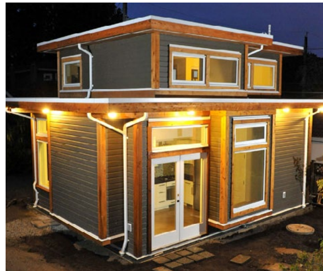
Figure 15: The second storey of a garden suite with a flat or shallow roof steps back and away from adjacent neighbours
